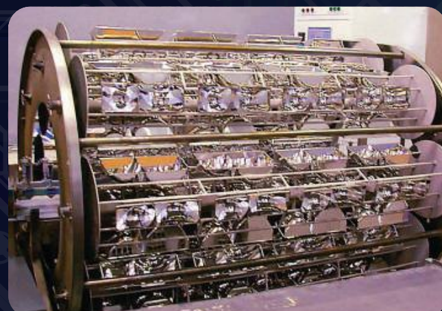
APPLICATION OF REFLECTIVE COATING ON RENAULT HEADLIGHTS
