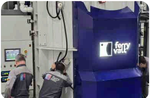
Coating system for large-sized products (up to 6 m) – VATT 5000-4M-S
