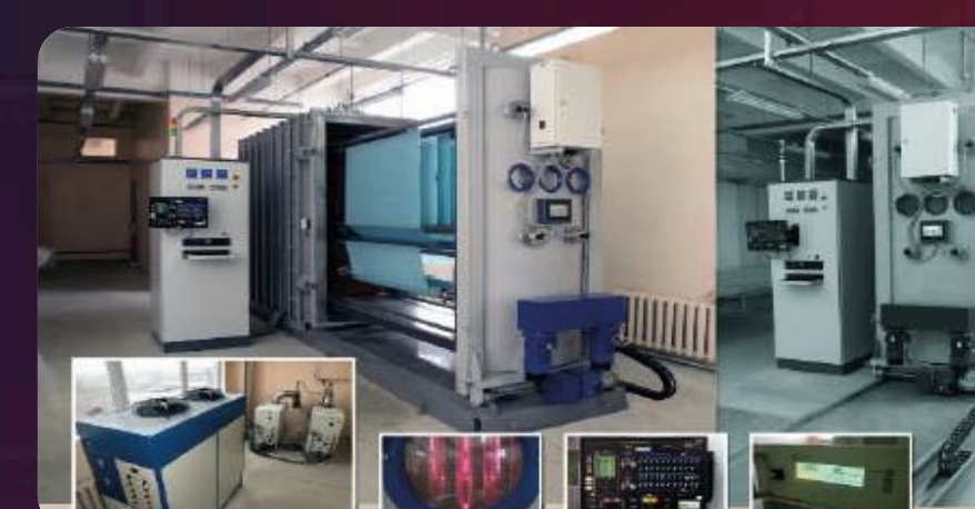
PLASMA ACTIVATION AND METALLIZATION OF FABRICS
