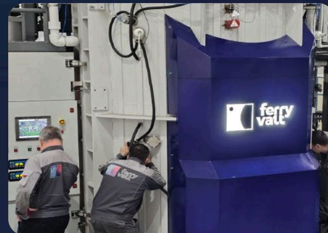
COATING SYSTEM FOR FUEL CLADDING TUBES (TVEL)
