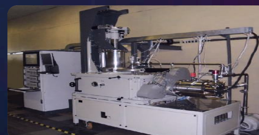
ELECTRON-BEAM DEPOSITION OF A WIDE RANGE OF COATINGS
