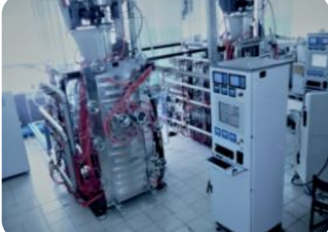
Series of zone melting systems for single crystals – VATT UZP-800
