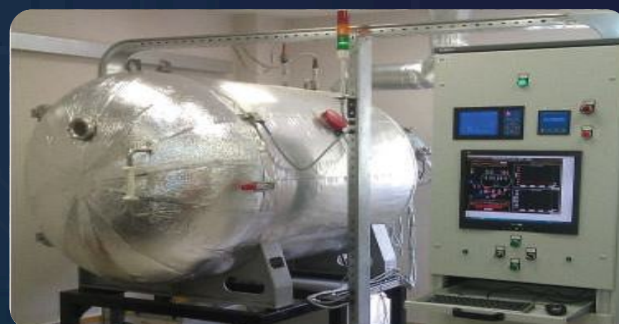
SPACE ENVIRONMENT SIMULATION FOR ROCKET-SPACE EQUIPMENT TESTING
