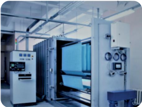
VATT 4000/5000 vacuum system series for roll-to-roll materials
